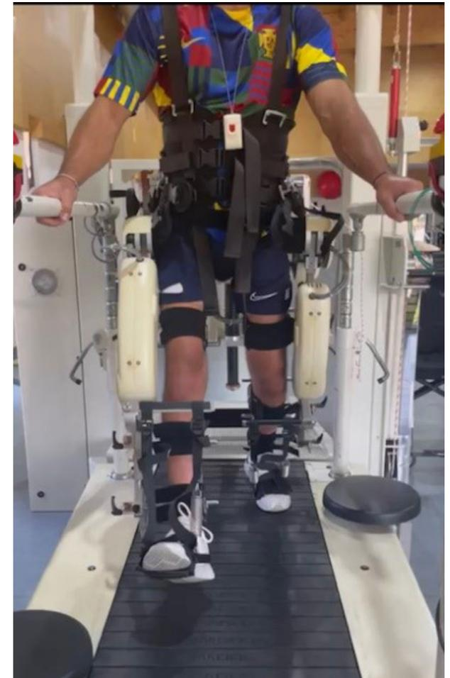
Figure 3: Lower limb rehabilitation exoskeletons (Source: authors)
