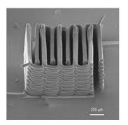
For the first time, a research team from the Wyss Institute at Harvard University and the University of Illinois at Urbana-Champaign demonstrated the ability to 3D-print a battery. This image shows the interlaced stack of electrodes that were printed layer by layer to create the working anode and cathode of a microbattery. [Ke Sun, Teng-Sing Wei, Jennifer Lewis, Shen J. Dillon] Credit: Wyss Institute
