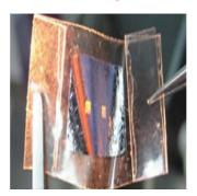
Flexible nanosensors which can adhere to biological surfaces such as human skin will improve the use of wearable devices that measure breath, heart pressure and temperature. The low-cost technology developed by researchers at the Universidad Politécnica de Madrid (UPM) Institute of Optoelectronics Systems and Microtechnology (ISOM) uses standard polycarbonate disks, adhesive tape and aluminum, which is 25,000 times cheaper than gold.
