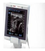
Esaote's MyLabTMOne Vascular is the first tablet-size ultrasound dedicated to vascular care. The system has a touch-screen display, interchangeable probes, long-life battery, internal archive and wireless connectivity for data sharing. In addition to high quality standard B-mode, Colour and Doppler it includes exclusive technology to measure intima media thickness (IMT) and arterial stiffness (AS) on the basis of radiofrequency signal analysis.
