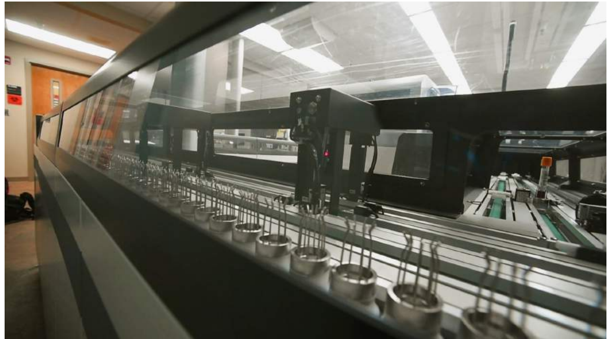
This moving track moves tubes of blood to the automated lab (Photo Credit: UAB)
