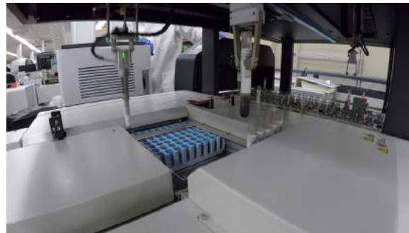
At the end of the line, small, grasping mechanical arms pick up the tubes and place them into refrigerators that can hold 10,000 tubes or into room-temperature storage for 5,000 tubes, in case further testing is needed (Photo Credit: UAB)
